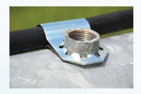
The Span Cable Clamp is installed using a specialty made tool also available from Reinke, wrapping tightly around the span cable, then slipping over the 3/4" sprinkler outlet coupler. The span cable should be installed with placement on alternating sides of the couplers for the Span Cable Clamp to work effectively. The Span Cable Clamp can be installed on each coupler, every other coupler, or on any number of couplers to customize the level of security.
